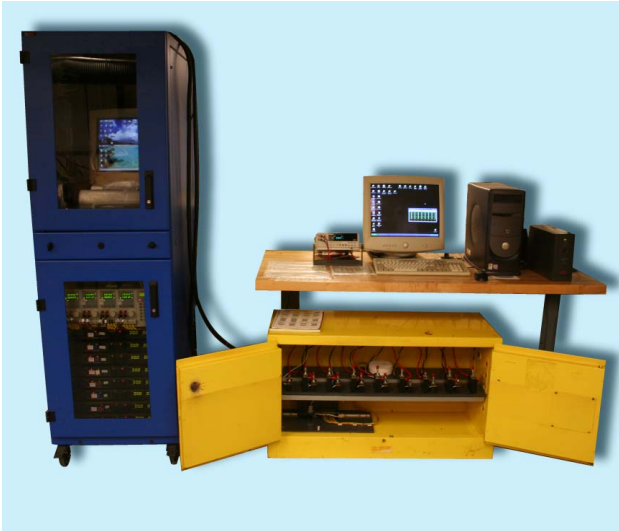
Figure 4. One of the automated test stands used for electrically qualifying cells, quanta, and bricks. Note the fireproof cabinet that contains the cells under test. Over 22,000 cells have been tested using such systems. To date, Bluefin Robotics has produced 165 pressure-tolerant batteries, with capacities ranging from 1.0 to 3.6 kWh.
