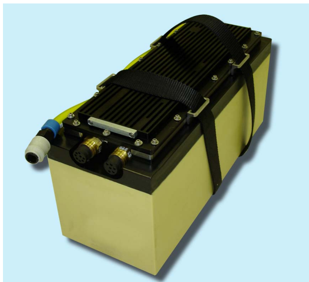
Figure 2. An older instantiation of the battery. Notice the plastic tube used for pressure-compensation and the need for pigtailed in the vehicle to mate with the battery connectors. Together, the pigtailed and tube occupied significant weight and space in the vehicle.
