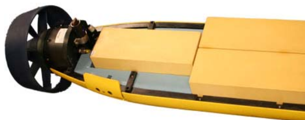
Figure 3. Rear section of the Bluefin 12" AUV. Three 1.5kWh batteries connect to the bottom mounted junction box to provide a uniform flat surface for floatation placement.
