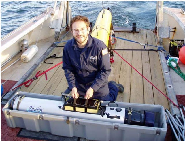
Figure 5. Bluefin's pressure-tolerant battery design and development program has yielded a COTS battery system that is used across the Bluefin fleet of 9", 12" and 21" AUVs in addition to third party ROVs and other systems. This picture demonstrates the ease with which a user can replace the battery in the Bluefin 9" (Sealion) AUV. Concurrently swapping the data module removes almost all of the delay normally associated with back-to-back missions.
