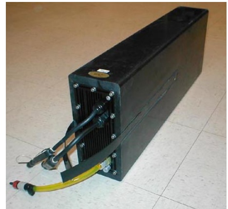
Bluefin 3.5 kWh Lithium-Polymer Battery
